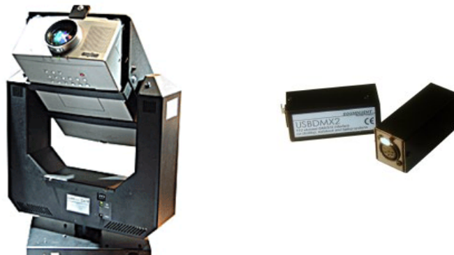
Figure 4.1: Left shows an example of the steerable projector unit [11] used in the system. Right shows the USB to DMX interface which is used to connect the projector to a computer [42]
