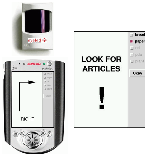
Figure 2. The hardware of the PDA-based shopping guide. (Left: Example display on the PDA, which receives location signals from a beacon (shown at the top). Right: Close-up of part of the display in the situation where the user has arrived at a relevant store.)
