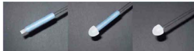
Figure 4: Differently shaped ends of the rods providing affordances for turning, pulling and turning, or just pulling
