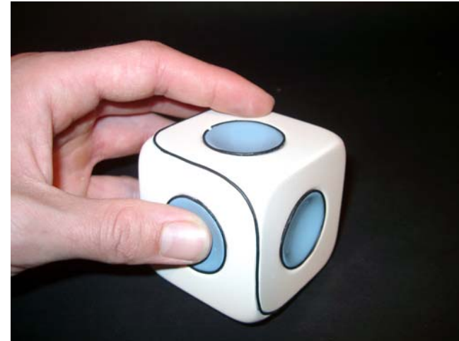
Figure 19: The final prototype of the cubical device, without labels for operational modes
