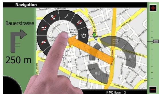
Figure 1. Pie sub menu for changing routing criteria of the navigation system. Appears when the user pulls his finger over the dedicated pie slice in the main menu and stops anywhere on the screen (location independent).
