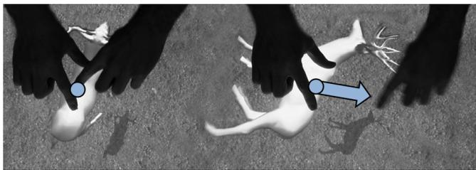
Fig. 2: Rotation technique described by Hancock et al. [9]. Flips a virtual object about the axis described by the first two touch points.
