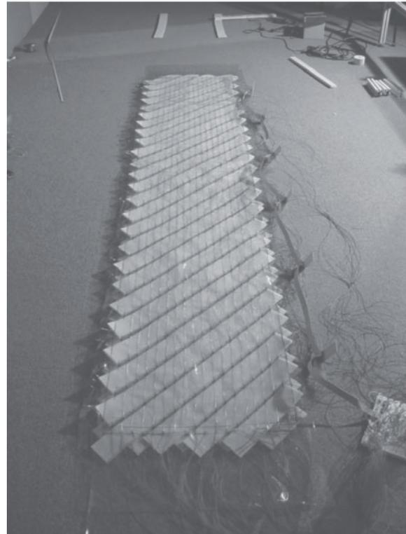
Fig. 7. Floor with sensors for gait recognition [30].
