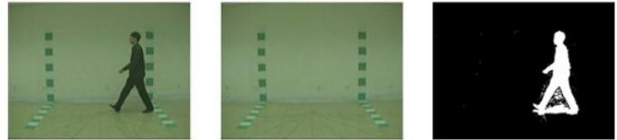
Fig. 6. Gait recognition based on video sensor using silhouette extraction [43].
