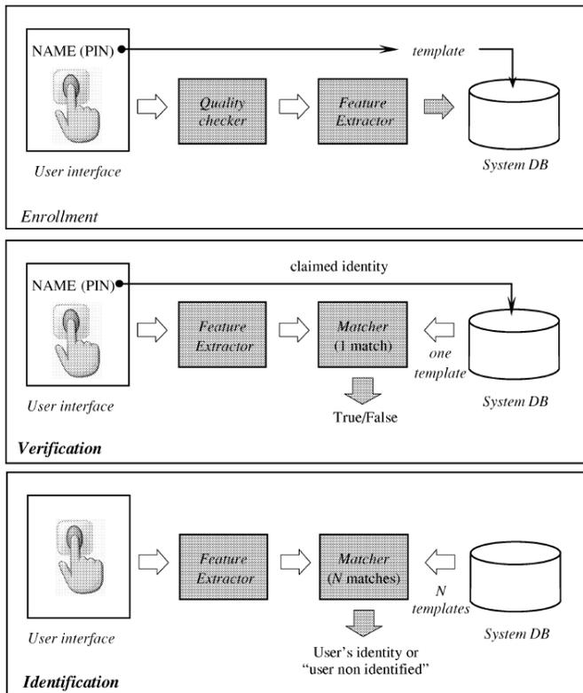
Fig. 2. Enrollment, verification and identification using the main units of a biometric system (sensors, feature extractor, matcher and database) [20].
