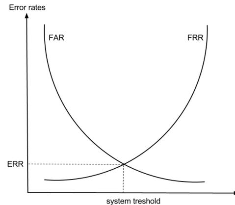
Fig. 3. Biometric system error rates.
