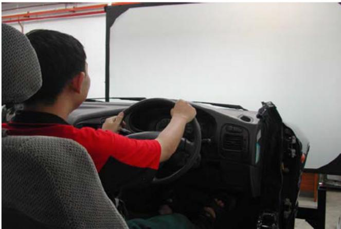
Fig. 2. Example of a driving cab in usage with Virtual Reality Technology [12]
