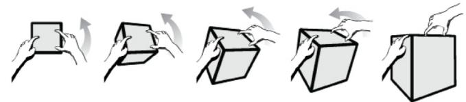
Fig. 3: Rotation technique described by Reisman et al. [19]: three fingers form a collinear configuration.
