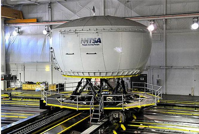
Fig. 5. Iowa Driving Simulator [14]
