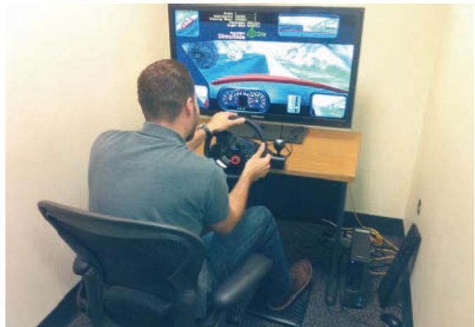
Fig. 3. Low fidelity driving simulator from Jeon [18]
