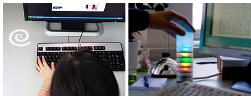
Figure 2. Left: The Ambient Appointment Projection projects calendar data onto the table. By a wiping gesture the user can acquire more details. Right: The StaTube shows the user's and contacts' IM states. By turning the upmost level the own state can be changed.
