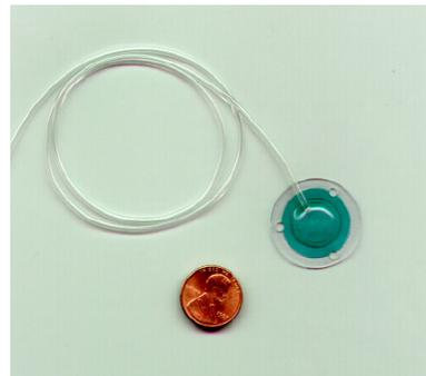
Fig. 8. Pneumatic tactile actuator [25]
