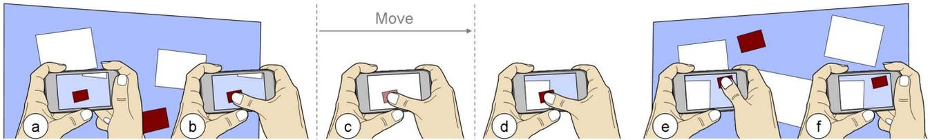
Fig. 7. Interaction with the *Touch Projector*: After aiming at the desired item (a), the user can select it by touching it (b). As the device leaves a display and moves off-screen, the item disappears and is displayed as a thumbnail (c). When the user reaches a second display, the dragged object reappears (d) and can be placed on its target position (e). It is dropped by lifting the finger (f). [6]
