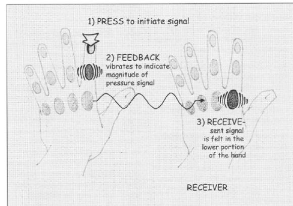
Fig. 6. ComTouch touch-to-vibration-mapping [2].
