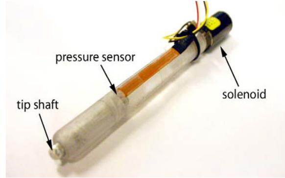
Fig. 13. Haptic Pen: Tactile feedback by means of a solenoid [15]
