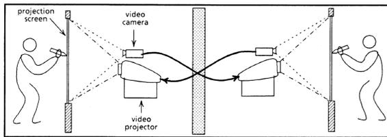
Fig. 2. Schematic of VideoWhiteboard system between two sites [6]
