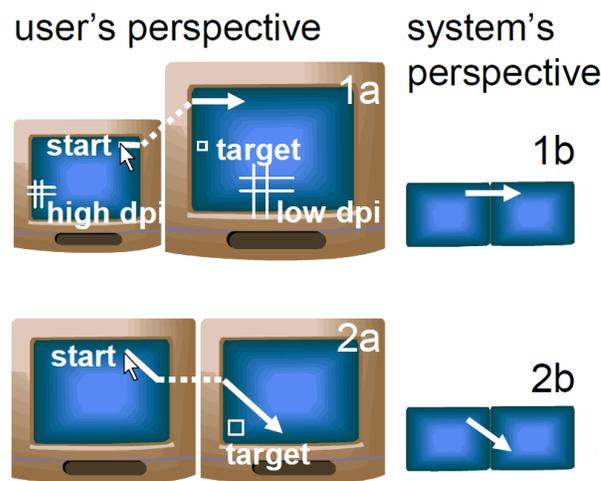
Fig. 2. Resolution (1) and offset (2) issues in a multi-monitor setup [3]
