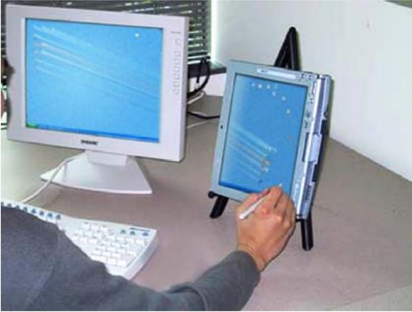
Fig. 5. *Drag-and-Pick*: Accessing content on an external monitor that does not support touch input [4]
