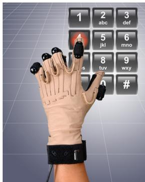
Fig. 9. CyberTouch: A CyberGlove with vibro-tactile feedback [7]
