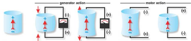
Fig. 7. Piezoelectricity [1]
