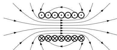
Fig. 3. Magnetic Field created by a solenoid [2]
