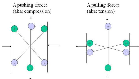
Fig. 1. the piezoelectric effect [1]
