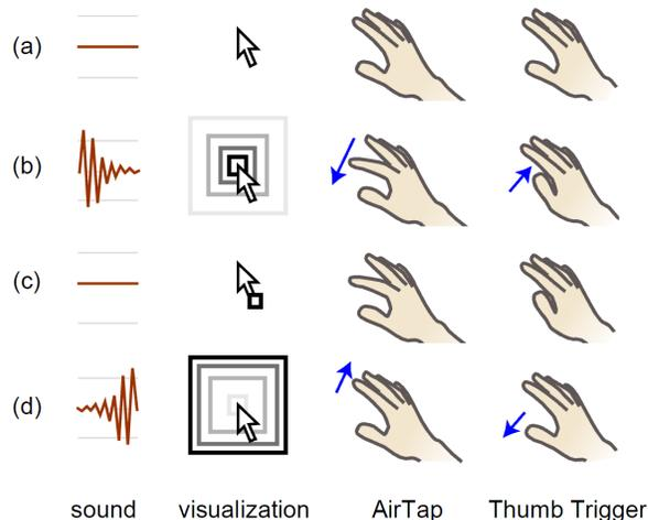
Fig. 6. The two clicking techniques *AirTap* and *Thumb Trigger* with their respective sounds and visual feedback. (a) shows the default state, (b) the click-down gesture, (c) the drag gesture and (d) the click-up gesture [20].
