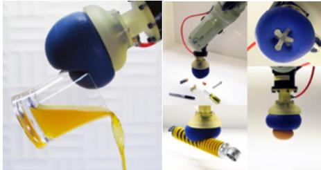
Fig. 4. A grasper using vacuum and granulate
