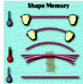
Fig. 6. Shape Memory Alloys [4]
