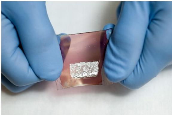
Fig. 8. A stretchable skin-like film developed at the Stanford University
