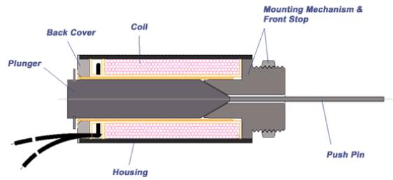
Fig. 6. Electromechanical push type solenoid [16]
