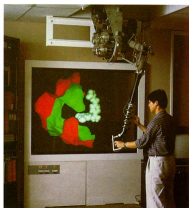
Fig. 4. The *GROPE-III* haptic display system by Brooks et al. [10].
