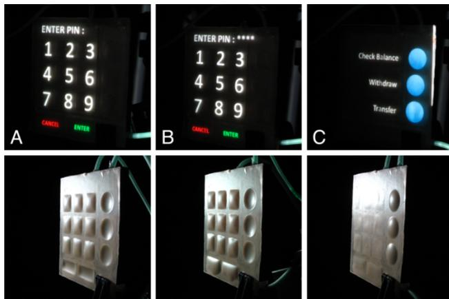
Fig. 17. Application example of the pneumatic display with different tactile configurations [10]
