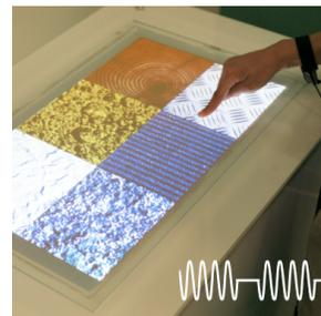
Fig. 19. TeslaTouch: Different texture and friction simulation [2]
