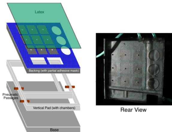
Fig. 16. Design example of a multi-chambered pneumatic tactile display [10]
