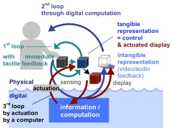
Fig. 2. The different interaction loops for TUIs with haptic/tactile feedback [11]
