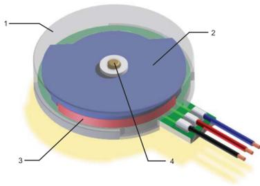
Fig. 4. "Coin-type vibration motor. A relatively flat eccentric weight spins in a protective enclosure. (1) enclosure, (2) rotor base, (3) weight, (4) shaft." [18]
