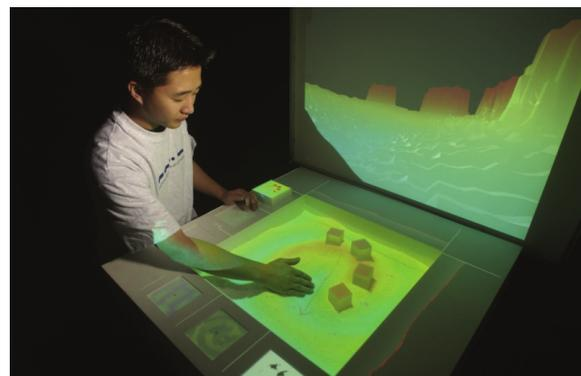
Fig. 1. SandScape: "Users alter the form of the landscape model by manipulating sand while seeing the resultant effects of computational analysis generated and projected onto the surface of sand in real time." [12]
