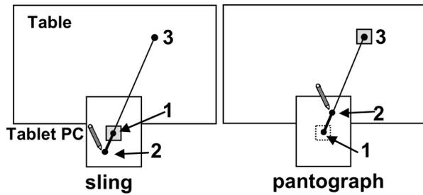
Fig. 3. *Slingshot* and *Pantograph*: (1) starting position of the object, (2) pen location for positioning the object and (3) target position of the object [11]
