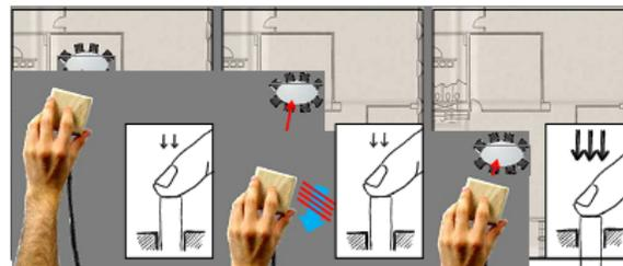
Fig. 1. HTP layout application: Moving an object inside the room with low pressure (left). Trying to move it outside its boundaries is not possible (middle) until enough pressure is applied (right) [8].
