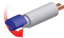
Fig. 3. Cylinder type vibration motor - an unbalanced weight is causing the device to vibrate [18]
