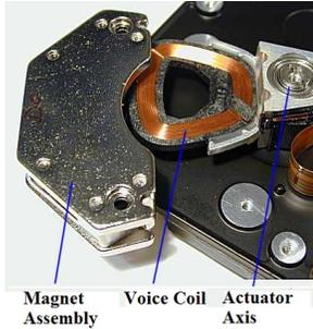
Fig. 4. hard disk using a voice coil as head actuator [20]
