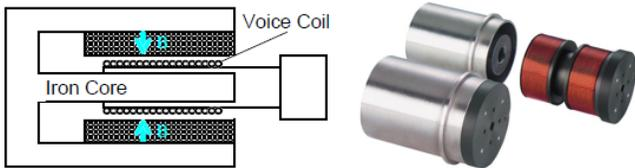
Fig. 5. Voice coil schematic (left); B is the magnetic field of the permanent magnet [26]. Example of a linear voice coil actuator (right) [3]
