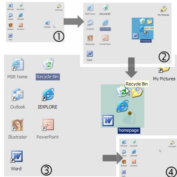
Fig. 1. The four steps of a *push-and-pop* [7] sequence: (1) The sequence is started by the user dragging a document. (2) The icons of compatible applications are displayed near the document. (3) The user drags the document over the recycle bin, which gets highlighted to show its selection. (4) The user releases the document and it is moved into the recycle bin.
