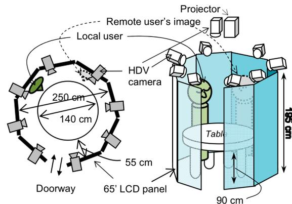
Fig. 3. Hardware Design of t-Room: Top-view (left) Bird's eye view (right) [8]
