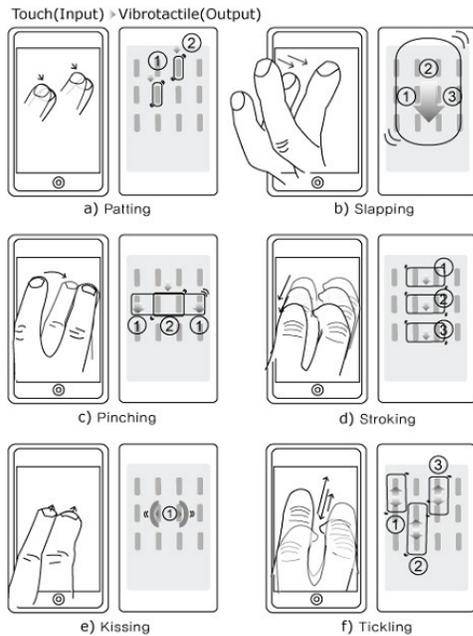
Fig. 8. CheekTouch: Mapping between touch input with fingers and vibrotactile feedback pattern on the cheek [9].
