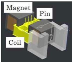
Fig. 5. Construction of a tactile display using voice coils
