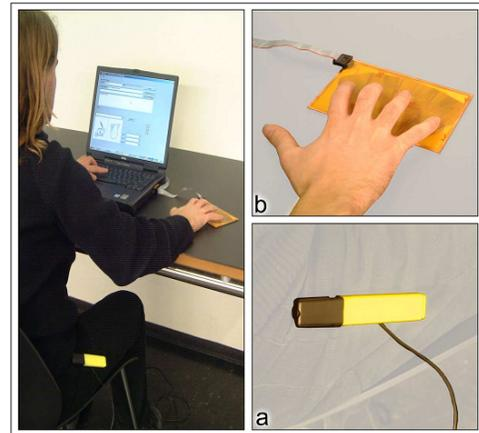
Fig. 7. HIM: Example of custom made devices: vibration device (a) and touch pad (b) [14].
