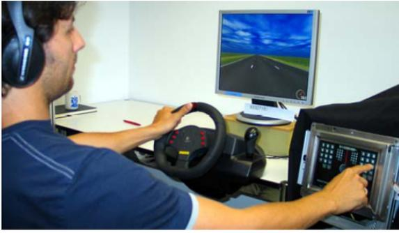
Fig. 11. "The HapTouch system is touchscreen device with tactile feedback" [22]
