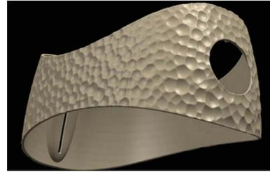
Fig. 7. The hammered surface of the virtual toaster created with haptic input [16].
