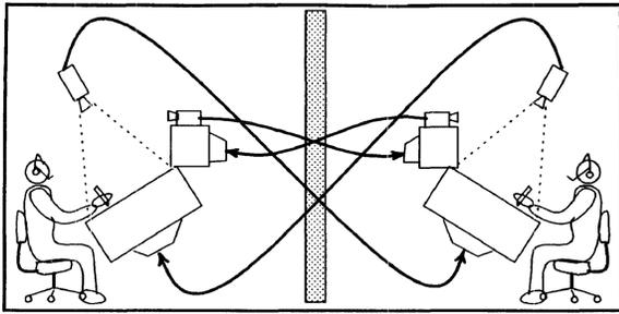
Fig. 1. Schematic diagram of 2 person videodraw [7]
