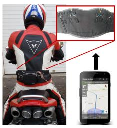
Figure 1. The MOVING system consists of a kidney belt with 12 integrated vibration motors controlled through a mobile phone application.
