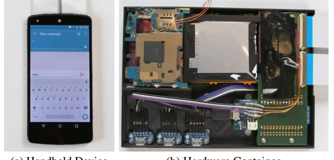
**Figure 2. Full-touch smartphone prototype:** (a) the *Handheld Device*, and (b) *Hardware Container* containing the processing units. Both components are connected via our self-designed PCB and flexible flat cables.
