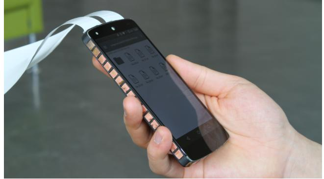
Figure 1. Our full-touch smartphone prototype based on two LG Nexus 5 and a Genuino MKR1000 for touch sensing on the edges.
