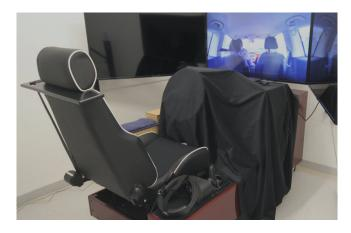
Figure 5: Our laboratory set-up consists of a driving simulator with a desktop PC, a display, and an Oculus Rift S headset (with a right-hand controller) connected to the desktop PC.
