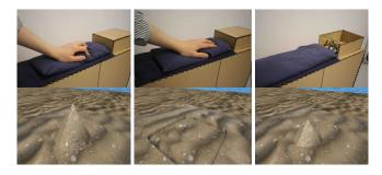
Figure 4: Our car-interior-based passive haptic display lets users feel and play with the sand while relaxing at a virtual beach during transit. Users can pile up (left) and push down (middle) the virtual sand. The images on the right show the user marks left on the interactive armrest and in the virtual sand.
