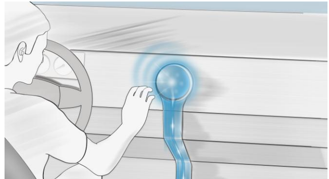
Figure 1. Heartbeat communicates the state of the electric drive and the batteries of EVs as visual and haptic feedback
