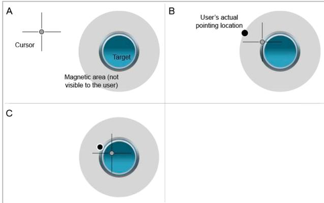
**Figure 2. The Magnetic Cursor. A: While outside magnetic areas, the cursor follows the user's pointing location. B: At the edge of a magnetic area, the cursor warps onto the corresponding edge of the target. C: When pointing closer to the target, the cursor moves closer to the target relative to the radius of the magnetic area and the distance between the actual pointing location and the center of the target.**
