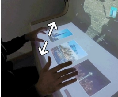
Figure 7 Example for concentrating the interaction on the horizontal display: zooming the map on the grey area with the left hand and dragging images with the right hand.
