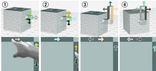
Figure 2. Extrusion workflow: arrows in the diagram indicate perspective-dependent polygon selections and the according gestures on the extrusion touch pad. (3) and (4): polygon selections flip when the view is rotated.
