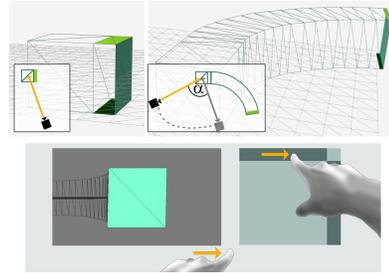
Figure 3. Creating bent shapes with simultaneous extrusion and camera control.  $\alpha$  is the angle of camera rotation and corresponds to the sum of rotation angles of the automatically extruded polygons.
