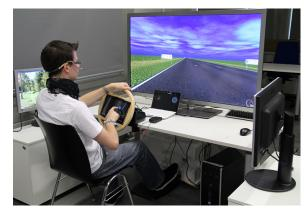
Figure 1: The study setup with multitouch steering wheel and speech input in the simulator.
