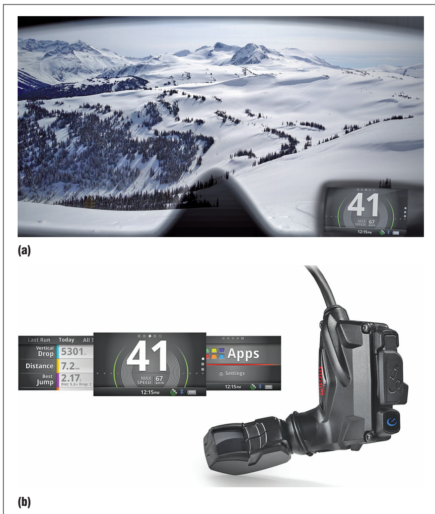
Figure 5. The Recon Instruments display can be used with (a) certain skiing goggles and shows current speed, altitude, and direction. (b) It can also display other information. (Photos courtesy of Recon Instruments; used with permission.)
