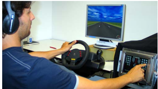
Figure 1: The HapTouch system is a force-sensitive touchscreen device with tactile feedback.
