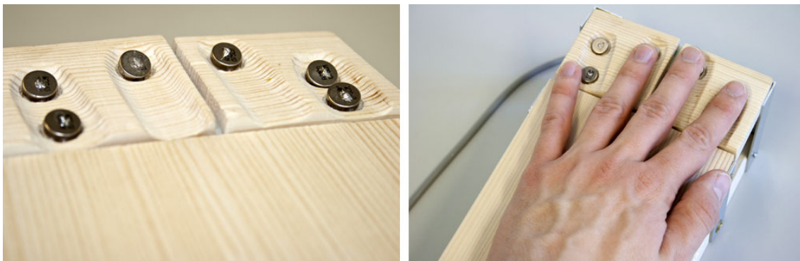
Figure 3: The Haptic Armrest. Left: two individually movable platforms and vibration actuators that are positioned under each fingertip. Right: the non-interacting hand is resting upon the actuators
