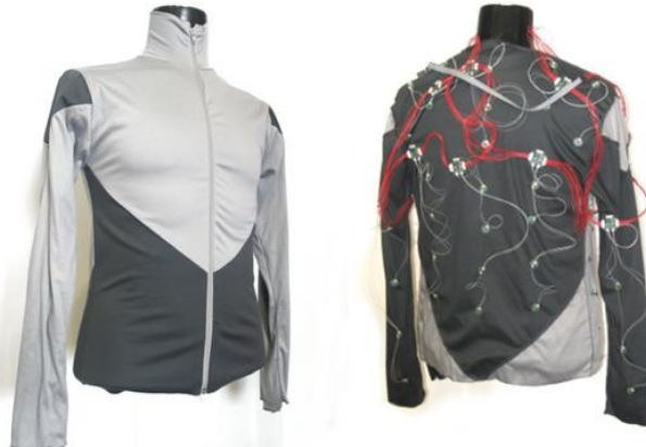
Figure 1. Outer lining (left) and jacket turned inside-out showing the inner lining with electronics and wires (right-hand panel). Red (thicker) wiring is the serial bus that connects all segment drivers and provides communication and power; white (thinner) wiring connects motor PCB's to the respective segment driver.
