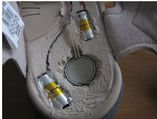
Figure 2: A picture of one pressure sensor and two actuators embedded in the shoes.
