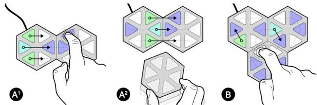
**Figure 5. This figure shows the transition-phase between two functionalities/modes (A/B) as well as the main input methods. Tapping on the device triggers mode-dependent actions (A<sup>1</sup>/B).**
