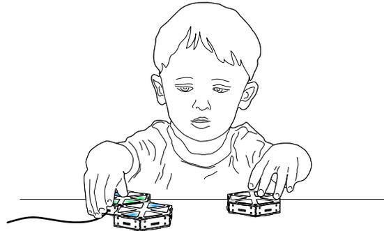
**Figure 1. The tangible modular interface COMB enables children to practice electronic/digital music. By building structures from block-like modules children can access different digital instruments. These instruments can then be step-sequenced<sup>1</sup> to create rhythms beyond the otherwise approachable complexity.**
