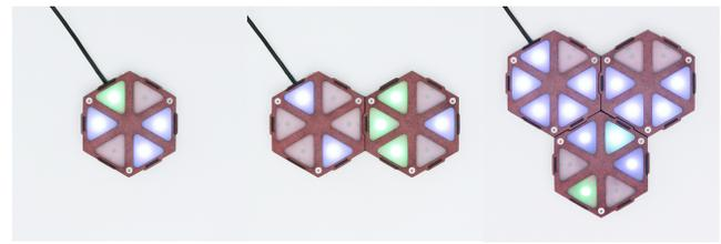
**Figure 4. Each shape represents an instrument/-group. The single element controls a kick-drum, two modules provide access to percussive sounds (snare, claps, rim), the triangular shape represents the opened and closed high-hat.**
