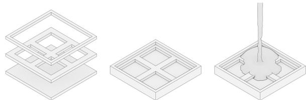
**Figure 8. A laser-cut-mold for custom silicone-pads can be manufactured from three simple layers of MDF. The middle layer defines the shape and number of pads, whereas the bottom and top layer restrict the flow of silicone.**
