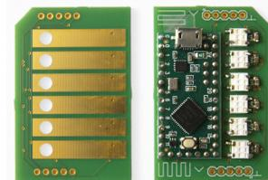
**Figure 10.** The prototype PCB shows that SMD parts are upside-down mountable which allows backlit-illumination through holes included in the PCB. Further, the possibility of the microcontroller SMD-style mounting has been proven to work seamlessly which reduces height requirements.
