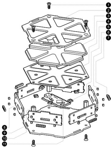
**Figure 9.** (1) screws, (2) top, (3) silicone-pad, (4) PCB, (5) WS2812b LEDs, (6) magnets, (7) spring loaded connectors, (8) flanks, (9) bottom, (10) spacer, (11) Teensy LC.
