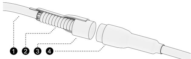
**Figure 7. A four-part structure has been used to overcome the loss of magnetic force caused by overheating magnets during soldering: (1) jumper wire, (2) ferromagnetic bridging-material (e.g. guitar strings), (3) magnet, (4) heat shrink.**
