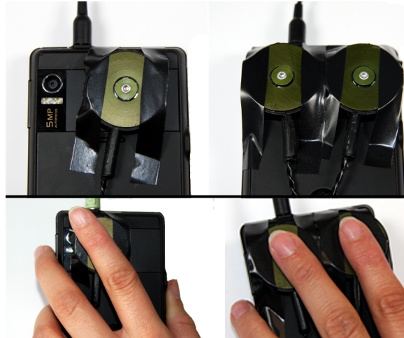
Figure 5.4 – Indoor study: Prototypes with one respectively two C2 tactors attached
