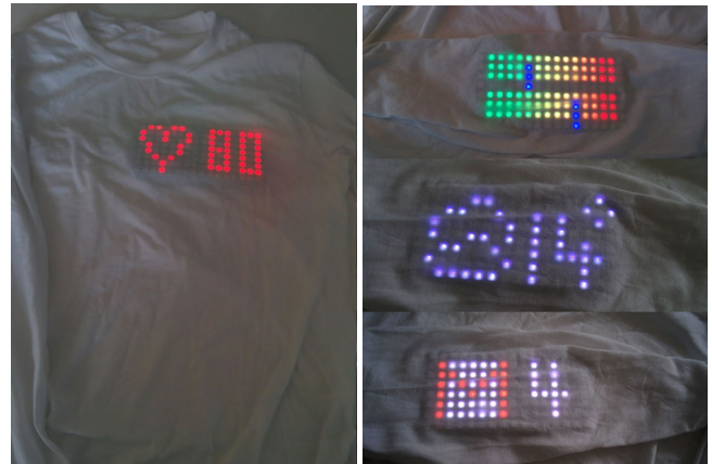
Figure 1. The wearable on-body display used in a t-shirt. The heart rate visualized on the chest (left) and a progress bar, weather information, and e-mail notification on the forearm (right).
