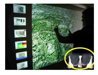
**Figure 1:** User is interacting with both hands and feet with a virtual globe using a large size multi-touch wall. User is standing on a Wii balance board (marked with yellow circle).
