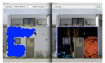
Figure 2. Programming the lighting controller of a retrofitted media façade by sketching the positions of the LEDs directly onto the architectural image [18].
