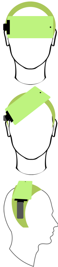
Figure 4: Illustration of the visor HMD design, a head-mounted display that slides up when not in use.
